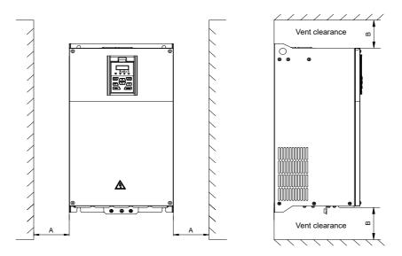
Fig. 3-3 Minimum mounting clearances of GK820-4T45D(H) and above
