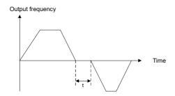
Fig. 6-11 Dead time between forward and reverse
