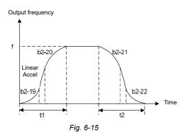
S-curve time at first segment of Accel is (b2-19×t1) in the figure, in which the Accel rate increases progressively. In this period, the S-curve time at last segment is (b2-20×t1) and the Accel rate decreases gradually. At the middle of t1, it is linear Accel with a constant rate which is adjusted automatically based on the setting of b2-19 and b2-20.
