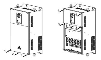
Fig. 3-10 Open the lower and upper cover
