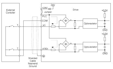
Fig. 3-17 Internal power supply dry contact
