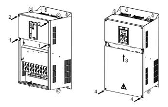
Fig. 3-11 Mount the upper and lower covers
