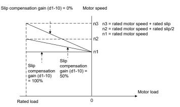
Fig. 6-45 Diagram of slip compensation on power generating load
