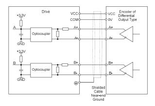
Fig. 3-30 Wiring of encoder of differential output type
