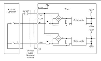
Fig. 3-18 External power supply dry contact
