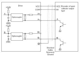
Fig. 3-26 Wiring of encoder of open collector output type
