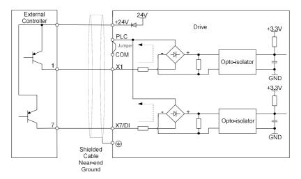
Fig. 3-21 Internal power supply open collector PNP connection
