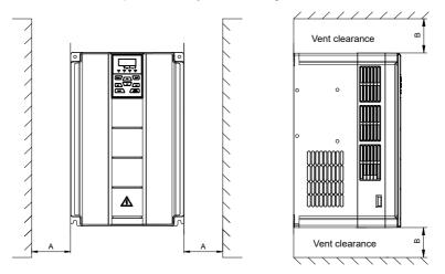
Fig. 3-2 Minimum mounting clearances of GK820-4T30(B/D/H)~ GK820-4T37(B/D/H)
