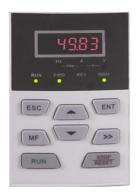
Fig. 4-6 Parameter setting status (b0-02 is set to 49.83Hz)
