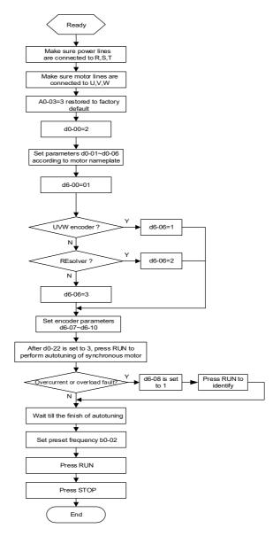
Fig.4-18 Flow chart of first-time power up for synchronous motor
