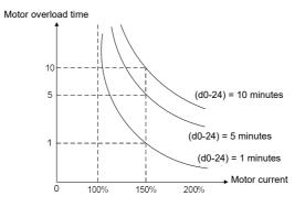
Fig. 6-39 Motor protection curve for ordinary motor running at 50Hz
