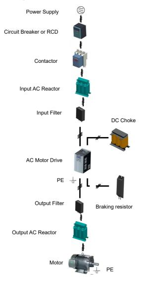
Fig. 3-12 Standard configuration of peripheral devices
