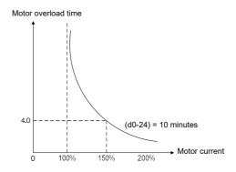
Fig. 6-40 Overload protection curve for ordinary motor running at 10Hz
