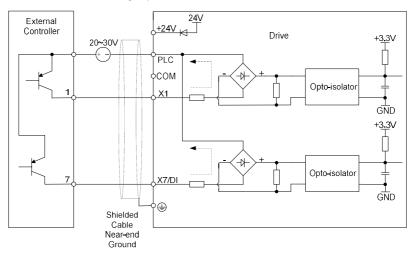
Fig. 3-22 External power supply open collector PNP connection
