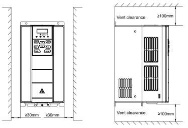
Fig. 3-1 Minimum mounting clearances of GK820-4T22B and below
