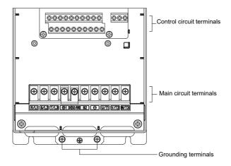
Fig. 3-13 Terminal configuration
