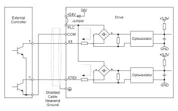
Fig. 3-19 External power supply open collector NPN connection
