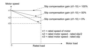
Diagram of slip compensation gain is shown as Fig. 6-44 and 6-45.
