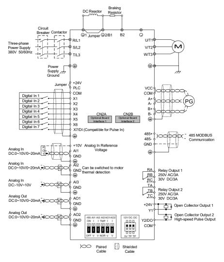
Fig. 3-15 Wiring diagram
