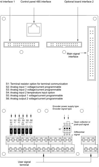
Fig. 3-14 Control board diagram
