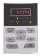
Fig. 4-7 Direct frequency modification status
