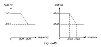
ASR parameters are normally adjusted in the following order: select appropriate switching frequency. Adjust proportional gain d2 -01 and integration time d2-02 at high speed, ensuring the system has no oscillation and meets the requirements of dynamic response characteristics. Adjust proportional gain d2-03 and integration time d2-04 at low speed, ensuring there is no oscillation at low speed and requirements of dynamic response characteristics are met.
