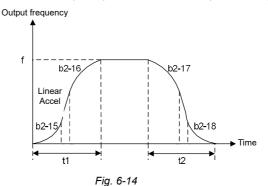
Accel/Decel rate changes gradually at the initial and ending segments of S-curve time. At the middle segment of S-curve, it is linear Accel/Decel rate, which is determined by enabled Accel/Decel time 1~4. Therefore, the actual Accel/Decel time is longer than linear Accel/Decel if this parameter value is selected.
