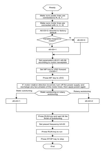
Fig. 4-17 Flow chart of first-time power up for asynchronous motor
