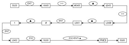
Fig. 4-15 Flow chart of locking control panel
