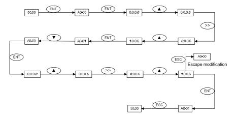
Fig. 4-11 Flow chart of user password setting
