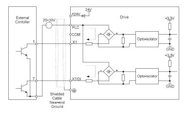
Fig. 3-20 External power supply open collector NPN connection
