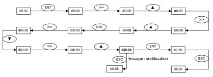
Fig. 4-12 Flow chart of upper limit frequency modification
