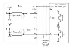
Fig. 3-28 Wiring of encoder of push-pull output type
